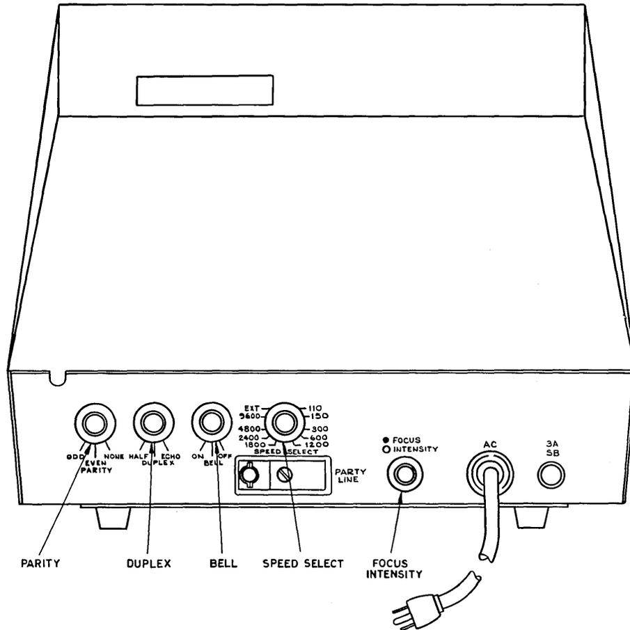
FIGURE 3-2. CONTROLS, REAR VIEW
