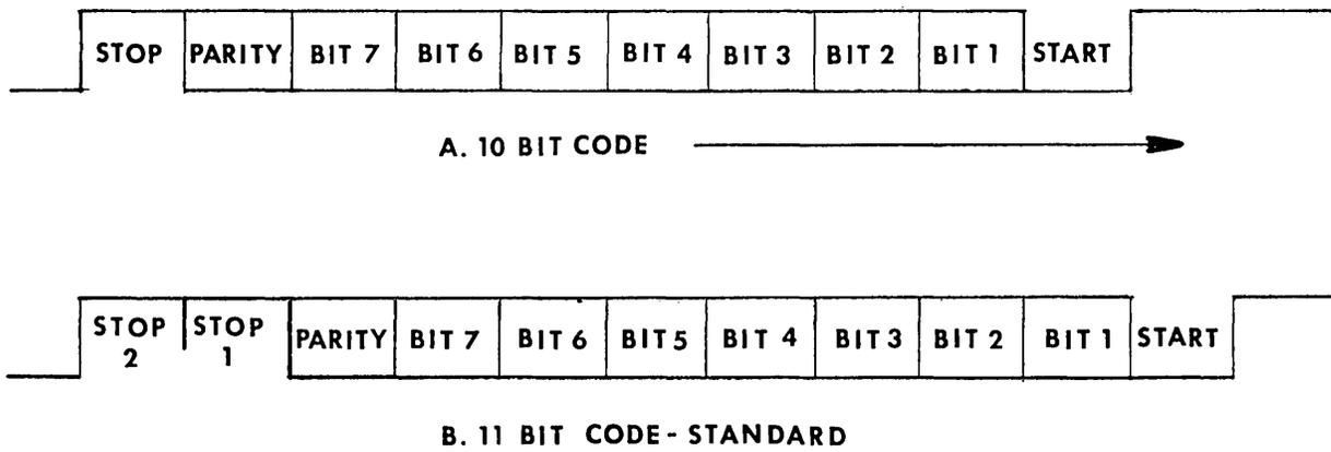
FIGURE 7-1 BIT SERIAL FORMAT
