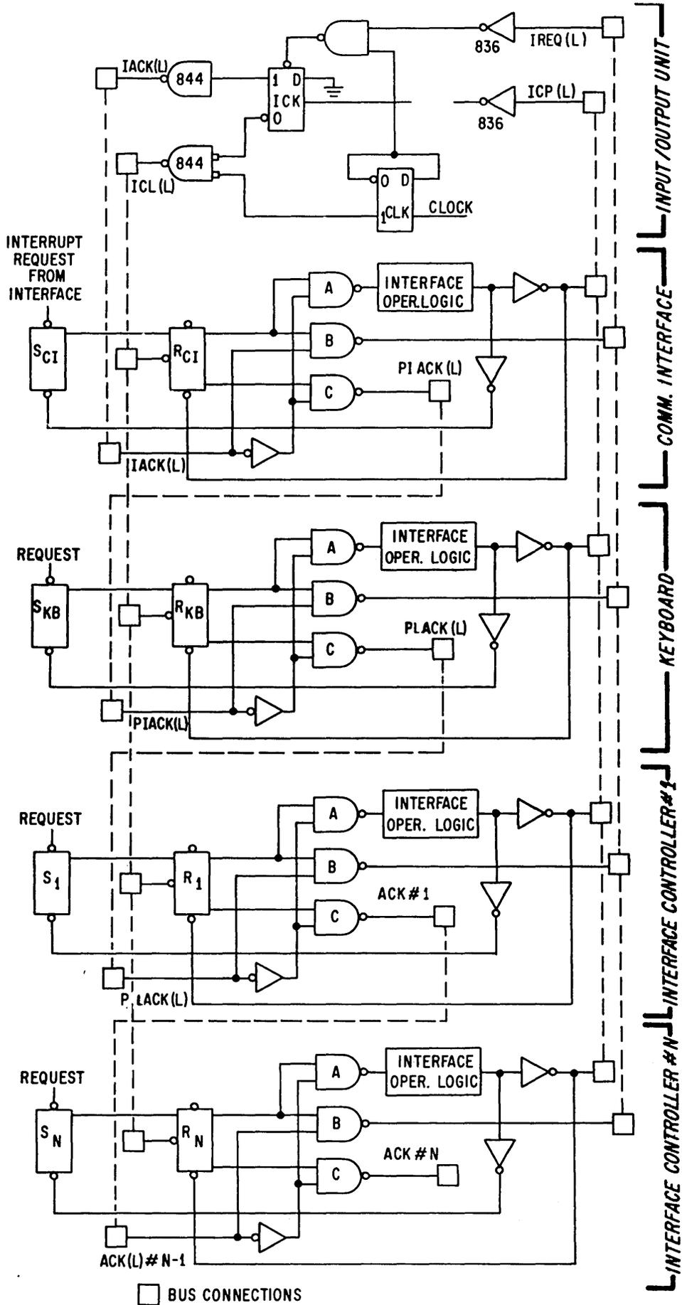
FIGURE 8-4 SEQUENTIAL PRIORITY INTERRUPT SCHEMATIC
