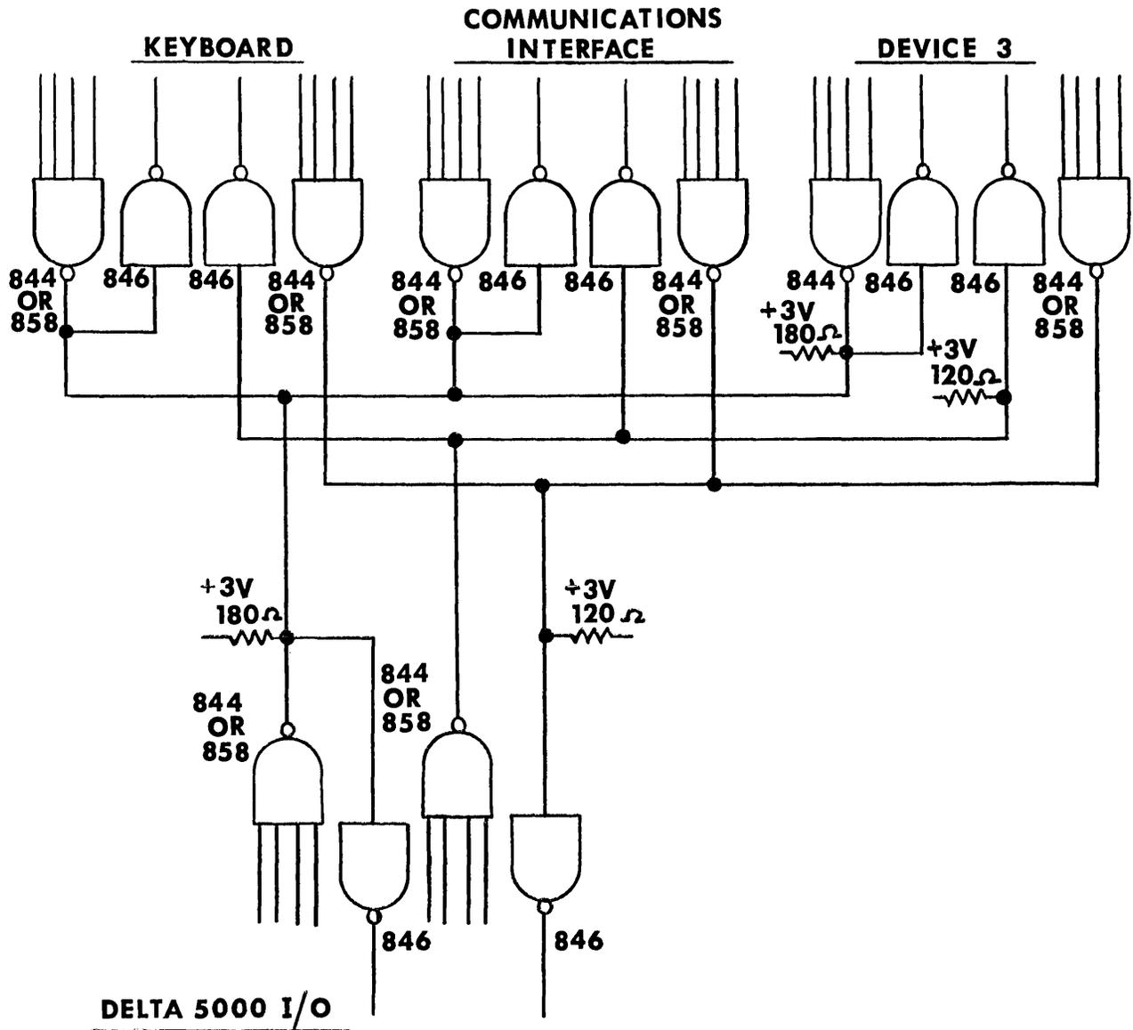
FIGURE 8-1 PARTY LINE LOADING INTERCONNECTING DIAGRAM
