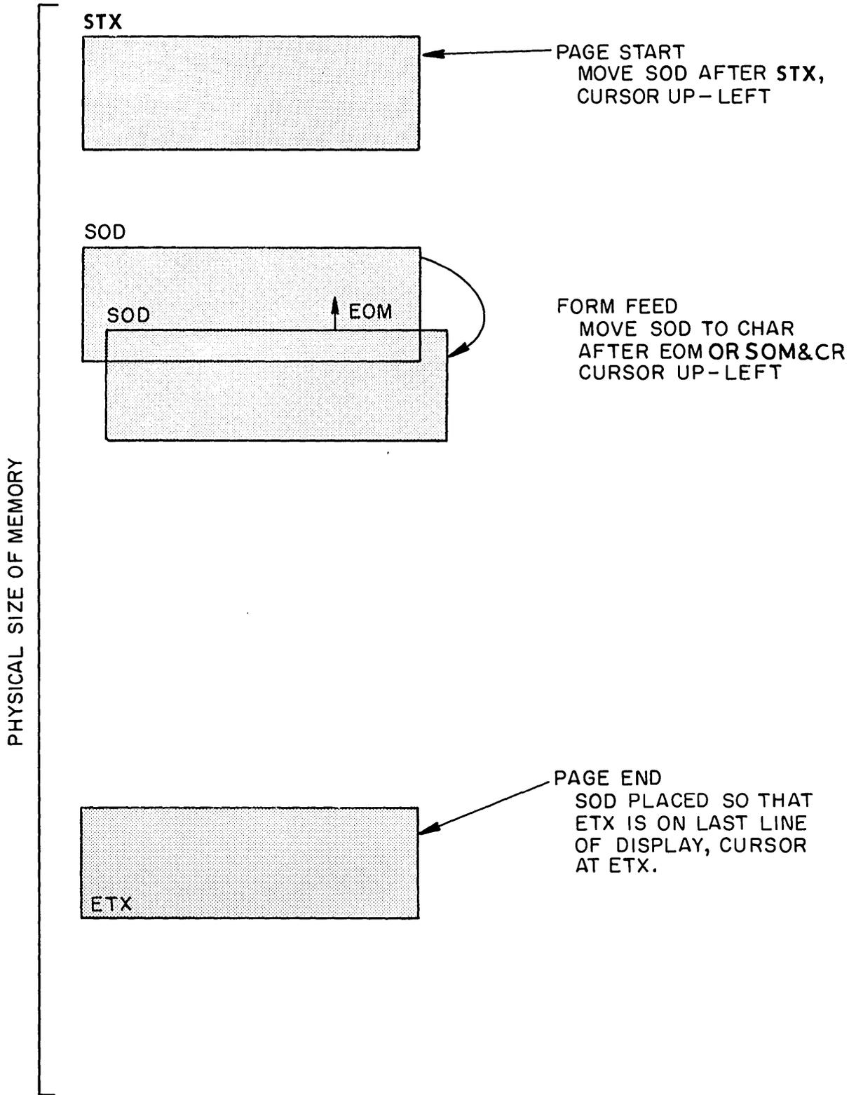
Figure 4-2 Example of Display Window
