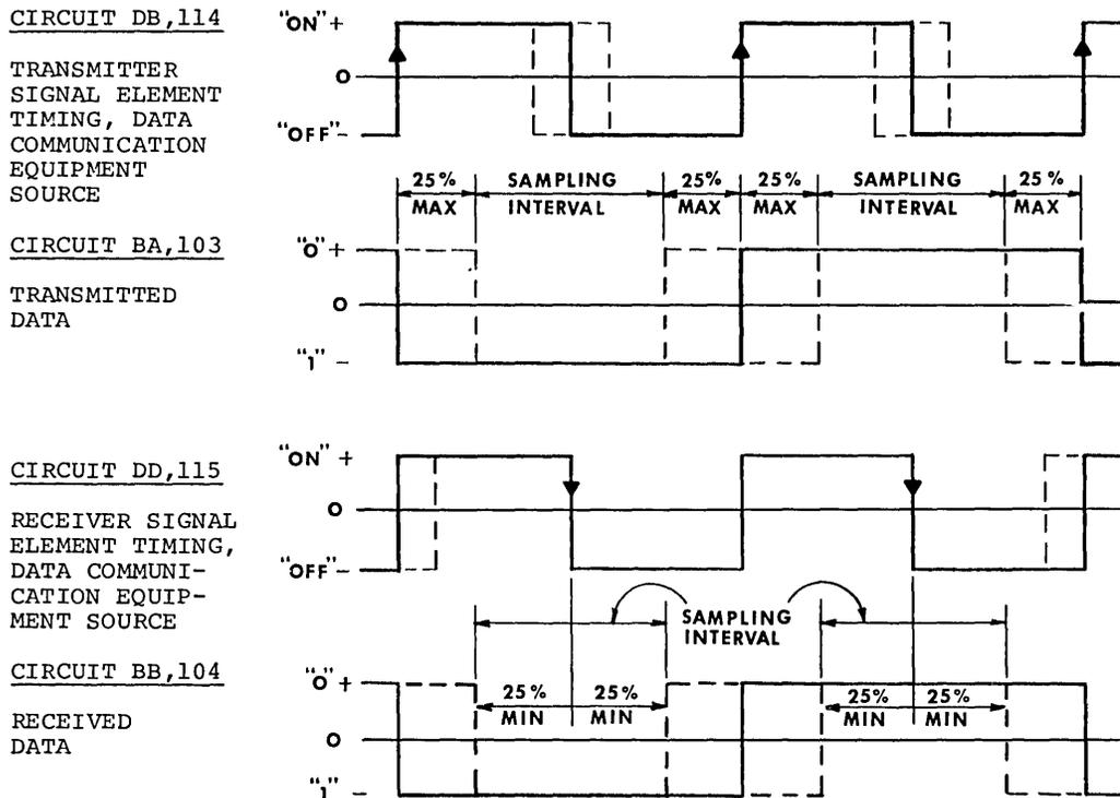
FIGURE 7-3. TIMING RELATIONSHIP BETWEEN DATA AND EXTERNAL CLOCKS
